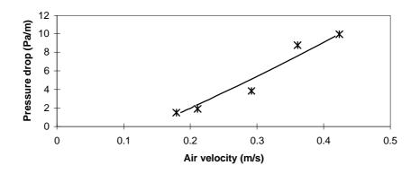
Fifure 6b. Comparison of pressure drop experimental data and model (17%wb)
