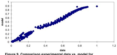
Figure 9. Comparison experimental data vs. model for thin layer drying of popcorn
