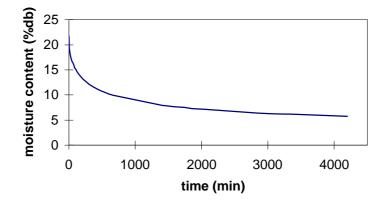
Figure 7. Thin layer drying of popcorn (run # 2)
