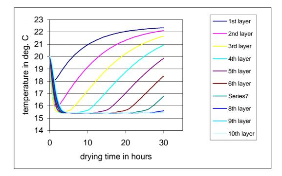
Figure 10. Predicted deep bed drying model for run No. 1
