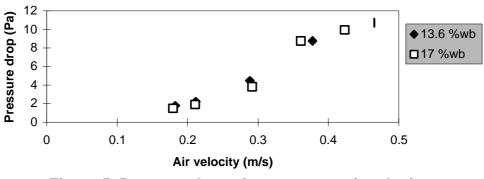
Figure 5. Pressure drop of popcorn vs. air velocity
