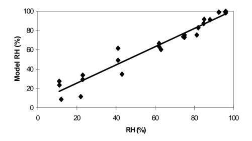
Figure 3. Chung-Pfost RH model
