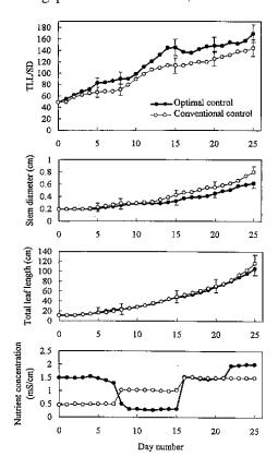
Fig. 6. Actual optimal control performance as affected by optimal 4-step setpoints of nutrient concentration.
