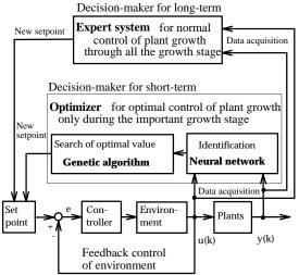
Fig 4 Hierarchical Intelligent control system composed of an Expert, a NN and a GA.
