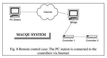
communication software to an IP bridge and gives control to the remote Macqu (Fig. 8), after level-access authorization checking. Further support is available for a camera connected to a Macqu controller to send images of greenhouse interior to the remote PC through Internet.
