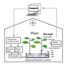
Fig 3 Hydroponic system control based on the SPA.
