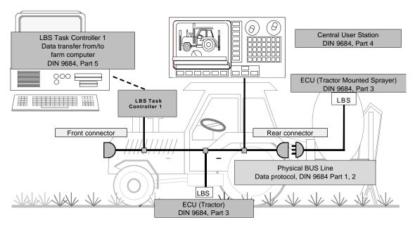
Fig 7: Scheme of a tractor-implement combination equipped with an LBS (source Speckman-FAL).
