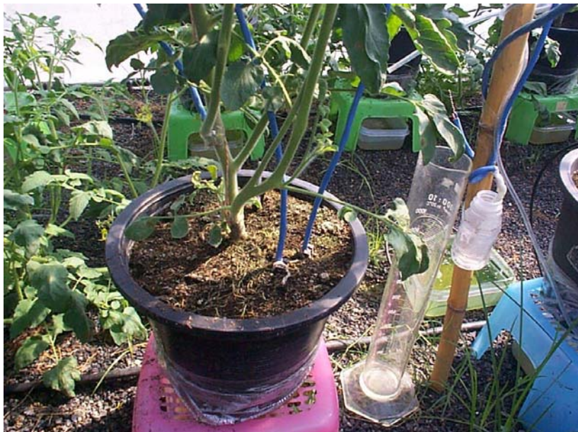
Figure 2. Soil temperature measurement at two depths (5 and 10 cm) and lysimeter arrangement for evapotranspiration measurement
