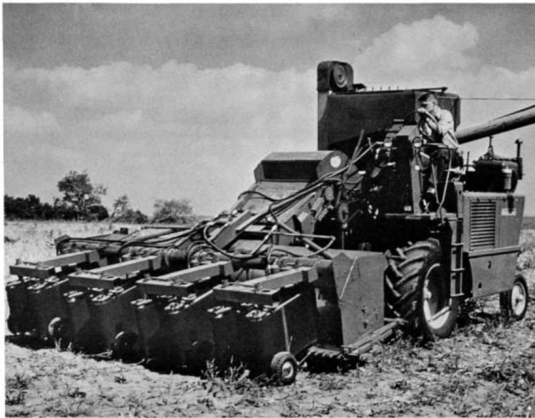
Figure 12. Bean combine with Cornell-developed direct-harvest pulling attachment.
