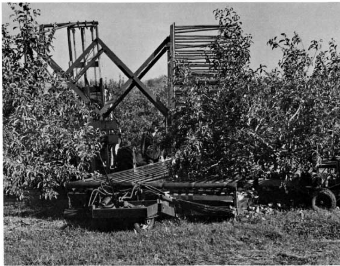
Figure 9. Padded tines are inserted into the tree near the fruit. These control fall of fruit from branches to catching frame. Fruit is detached by shaking either limbs or trunk.
