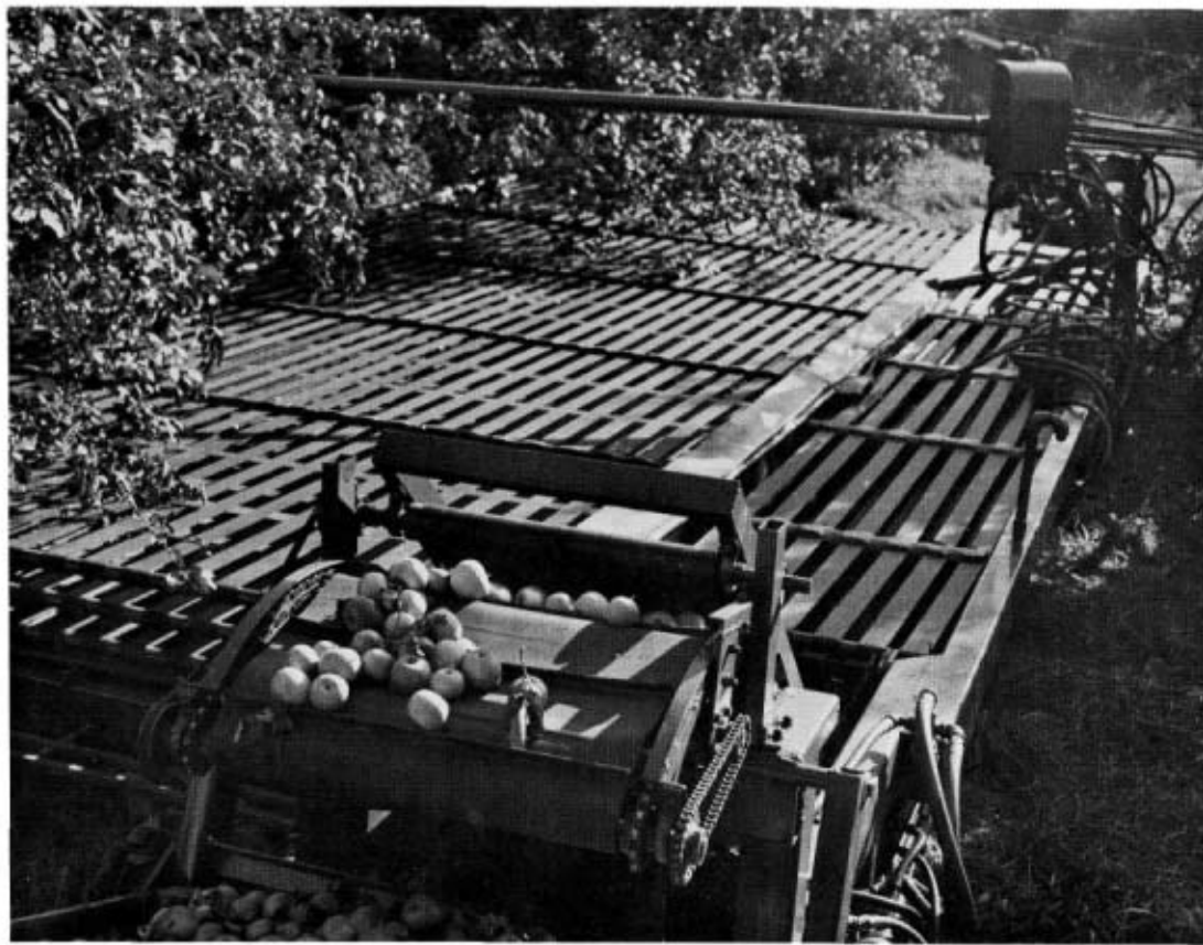
Figure 8. Close-up of the "output end" of the Perry apple harvester.
