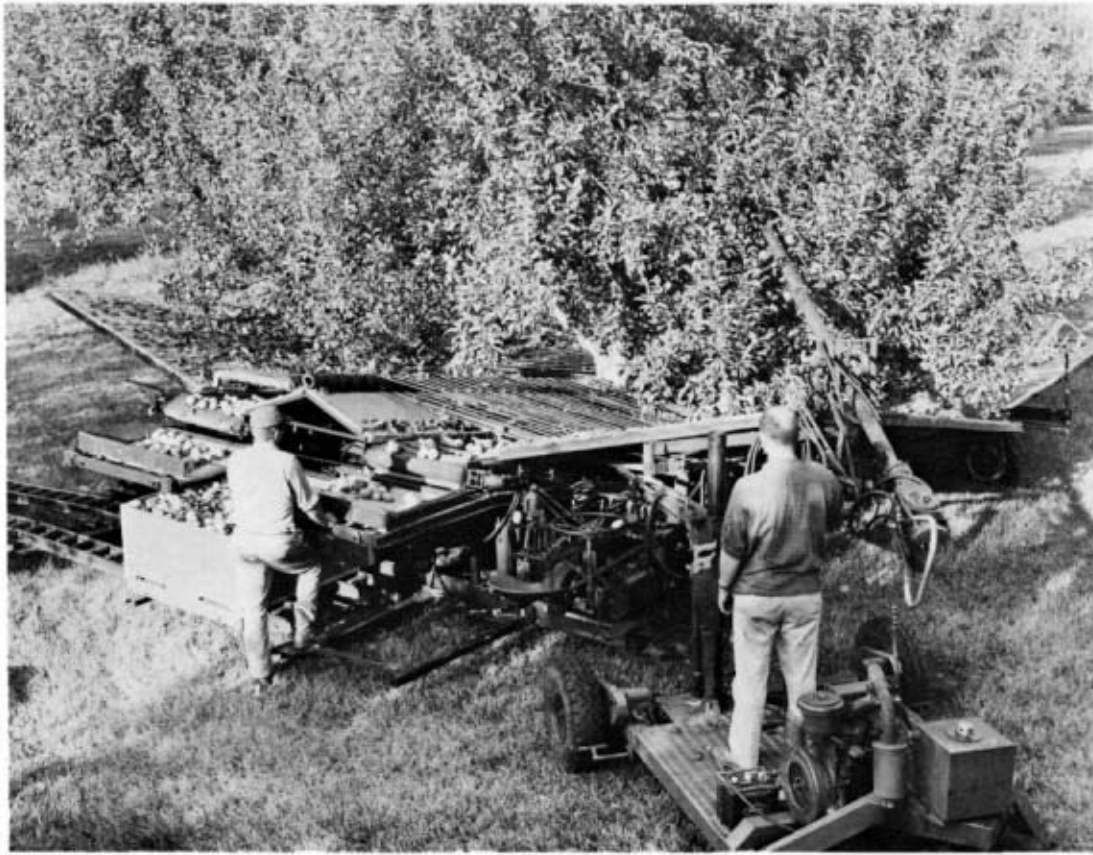
Figure 6. In early attempts to harvest apples mechanically, the Cornell cherry harvester was modified to handle processing varieties of apples.
