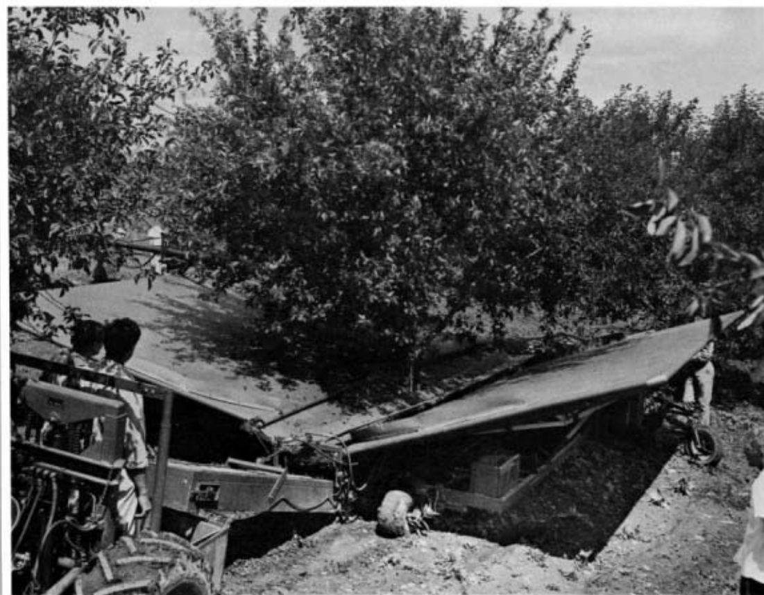
Figure 5. The basic concept for collecting cherries was developed from this experimental machine.
