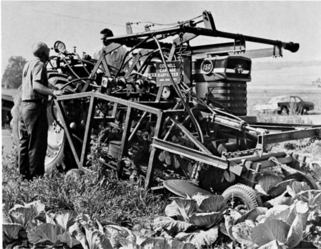
Figure 14. Entrance or "finding" discs, elevating-lifting conveyor, and re-orienting unit can be seen in this field picture of the cabbage harvester.
