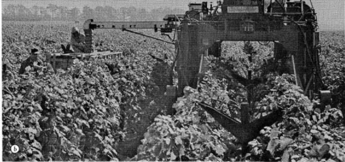
Figure 2(a). Diagrammatic sketch of Concord vines trained to GDC system. Spurs and canes are shown only on the middle vine of the post length. (b). 1967 CRCO spiked-wheel, vertical-stroke grape harvester, shown harvesting GDC-trained vines. Plastic-lined wood pallet boxes of 1-ton capacity in next row.
