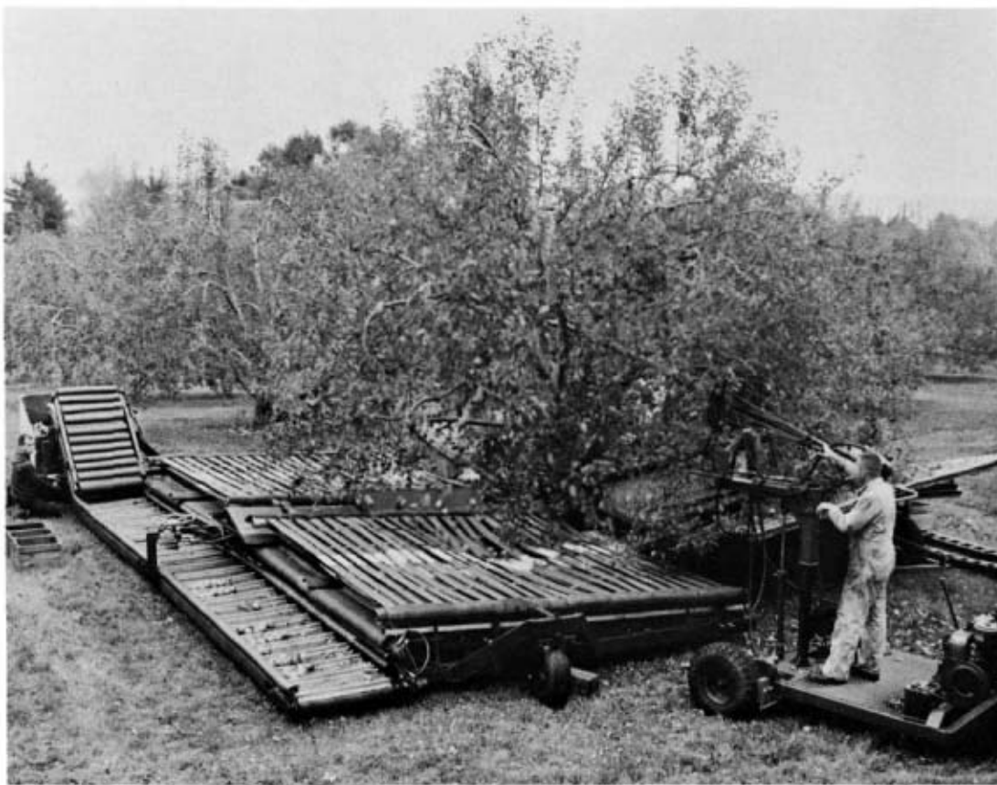
Figure 7. Field-testing the Cornell low-profile experimental multifruit harvester. Previous "apple version" of the cherry harvester at right.
