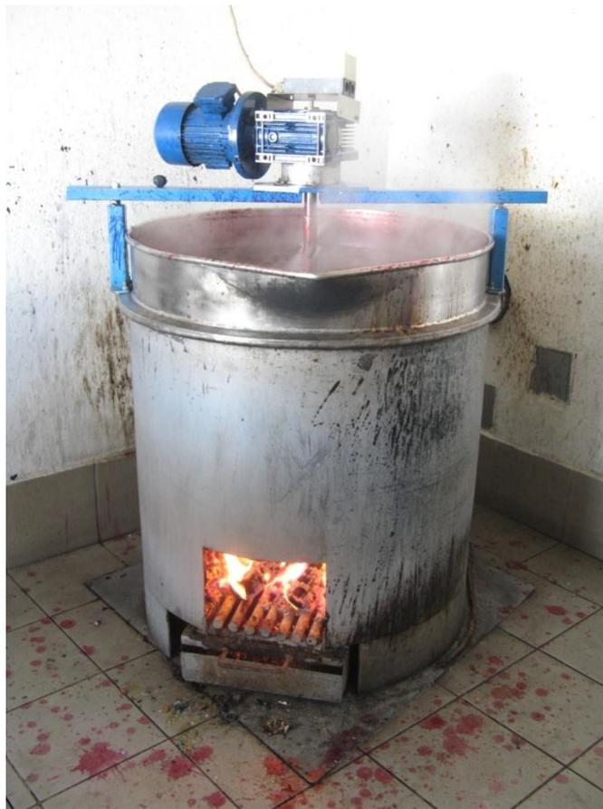
Figure 10. Motorized stirring pot. Photograph by Olivia Hall
