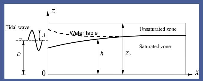
$$\frac{\partial \theta}{\partial t} = \frac{\partial}{\partial x} \left[ K(\psi) \frac{\partial \Phi}{\partial x} \right] + \frac{\partial}{\partial z} \left[ K(\psi) \frac{\partial \Phi}{\partial z} \right]$$
