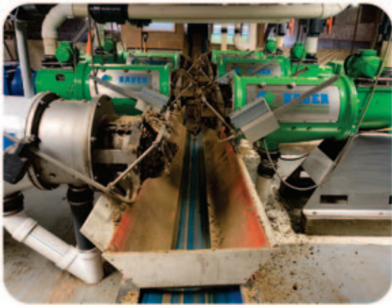
Successful screw press solid liquid separation system providing 60 percent dry matter solids for bedding from anaerobic digestate.
