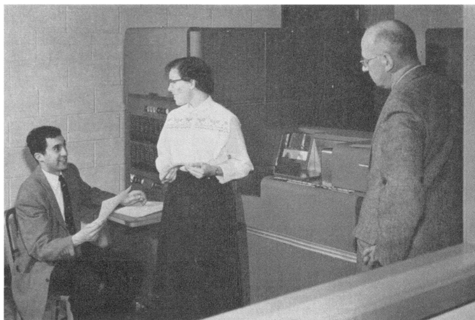
New "Brain" for Computing Center —Director Richard C. Lesser of the Cornell Computing Center, Research Assistant Virginia A. Walbran '52, and Professor Robert J. Walker, Mathematics, are pictured with the Center's new electronic brain, a 650 Magnetic Drum Data Processing Machine capable of 100 arithmetical operations a second. Cost of the machine was partly met by its maker, International Business Machines Corp. The Center has received $50,000 from National Science Foundation to furnish free computing services to University students and Faculty doing non-sponsored research. Photo Science
