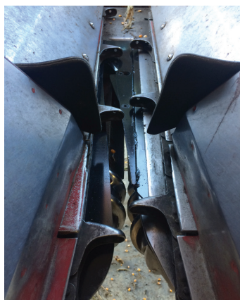
Fig. 5. “Sunflower plates” bolted on to the corn head keep the sunflower heads from bouncing forward and out.
