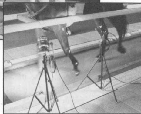
(Above) High-speed cameras record limb movement of a horse on the treadmill. (Right) Markers on the horse's limbs aid researchers in tracking limb movement
