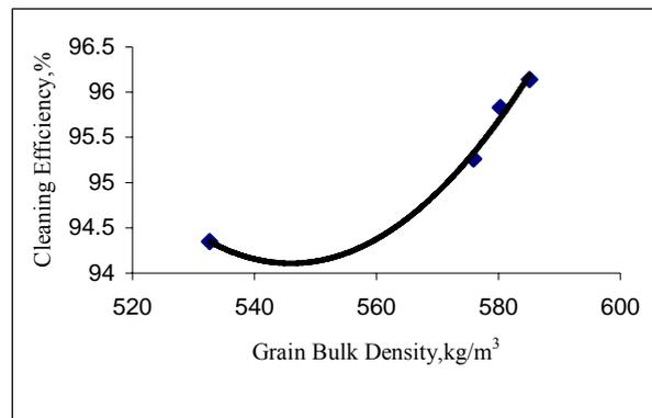
Figure 2: Effect of grain bulk density on cleaning efficiency
