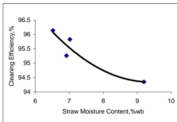
Figure 5: Effect of straw moisture content on cleaning efficiency.
