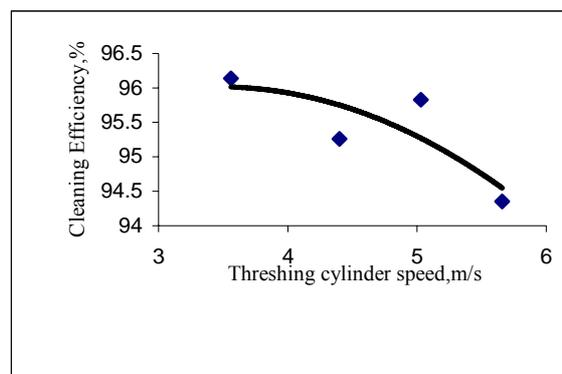
Figure 6: Effect of threshing cylinder speed on cleaning efficiency
