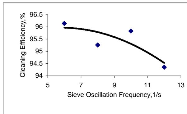
Figure 8: Effect of sieve oscillation frequency on cleaning efficiency
