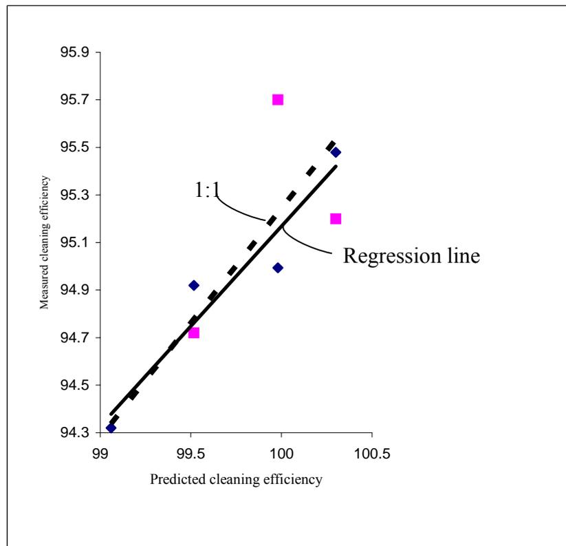
Figure 10: Plot of measured against predicted cleaning efficiency
