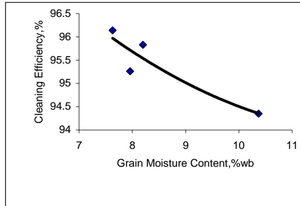
Figure 4: Effect of grain moisture content on cleaning efficiency
