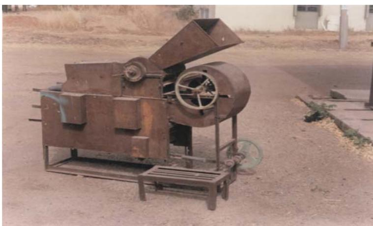
Figure 1: Side view of the sorghum thresher testing-rig
