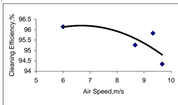
Figure 7: Effect of air speed on cleaning efficiency
