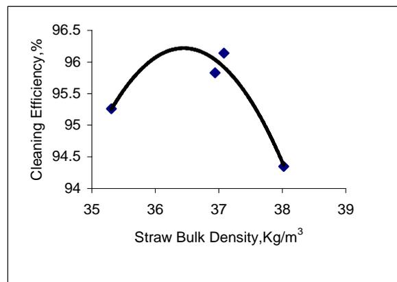
Figure 3: Effect of straw bulk density on cleaning efficiency
