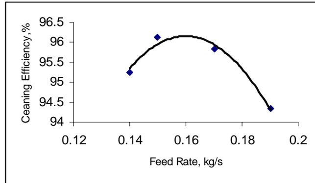
Figure 9: Effect of feed rate on cleaning Efficiency
