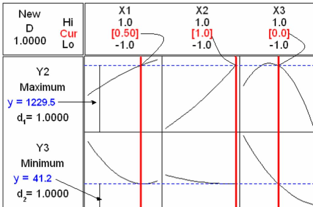
Figure 3.  $X_1 = 0.5, X_2 = 1, X_3 = 0$  Optimal solution (indicated in horizontal axis), for the two responses  $Y_2 = 1229.5, Y_3 = 41.2$ . The vertical axis displays the value 1 for desirability function  $d_1$  and  $d_2$ .
