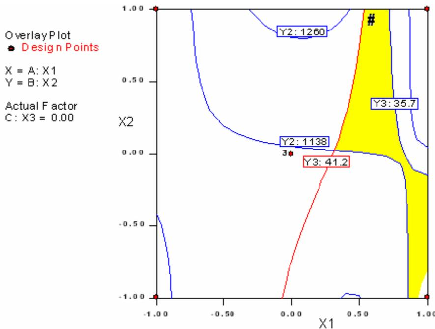
Figure 4. Contour plot superimposed for the variables  $Y_2$  and  $Y_3$ , the shady area describes a set of possible solutions with  $X_3 = 0$ .
