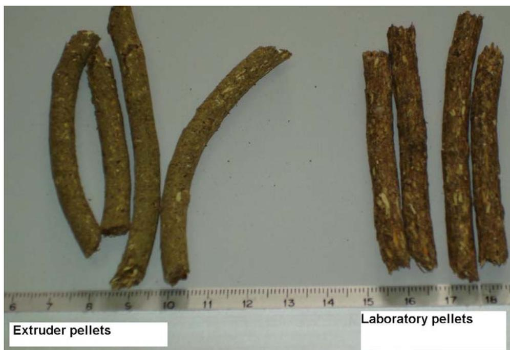
Figure 6. Comparison of pellets from the full scale extruder and from the laboratory.
