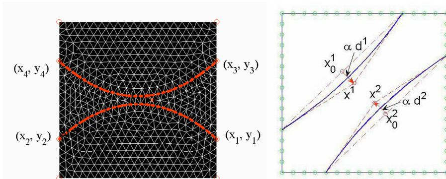
**Figure 2: End point co-ordinates of curvilinear stiffeners on EBF3 panel (left), and shape design parameter  $\alpha$  controlling the motion of the two mid points  $X^1$  and  $X^2$**
