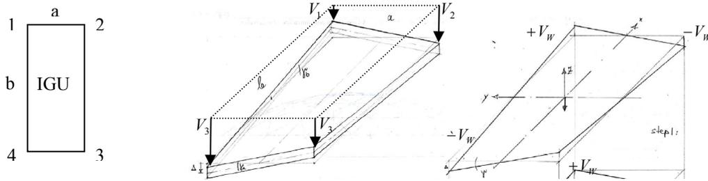
Figure 2: Calculation of total warping
