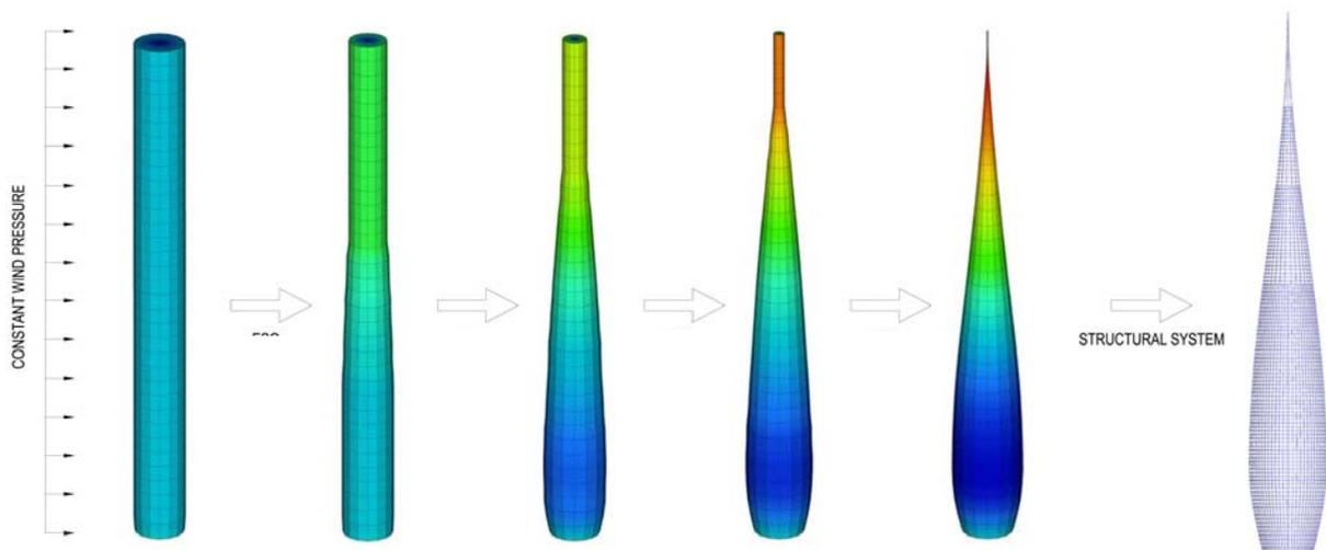
Fig. 3: Evolution of building shape to optimally resist lateral wind pressure.
