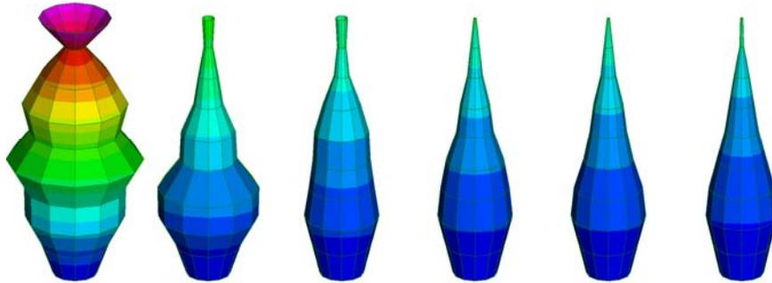
Fig. 4: Evolution of building shape using genetic algorithms.
