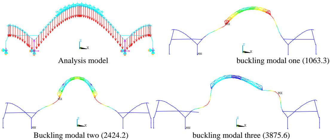
Fig.4 case1 buckling mode
