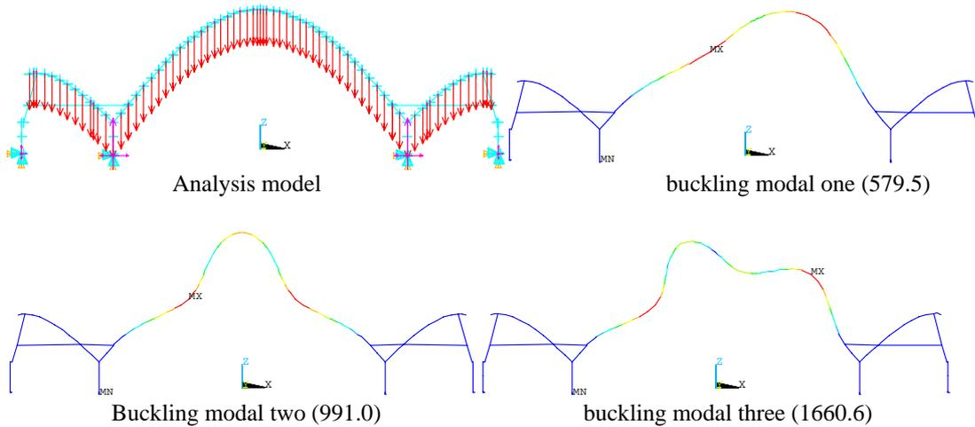
Figure.3 case1 buckling mode
