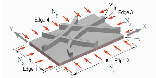
**Figure 1: Bi-normal load:  $N_x = 250\text{kN/m}$ ,  $N_y = 50\text{kN/m}$ , uniform vertical pressure:  $p = 10000\text{N/m}^2$ , fixed: edges 1 and 4, simply supported: edges 2 and 3, all aluminum  $a = b = 2.54\text{m}$ , with displacement constraint  $= \pm 0.1\text{m}$ . Initial size and bounds:  $t_0 = w_0 = 0.005\text{m}$ ;  $h_0 = 5w_0$ ;  $tb = wb = [0.0001, 0.1]\text{ m}$ ;  $hb = [0.0001, 0.5]\text{ m}$**
