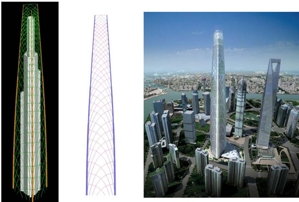
Fig. 2: Definition of the lateral system for a high rise by principal stress trajectories (left) and architectural rendering of the building (right).
