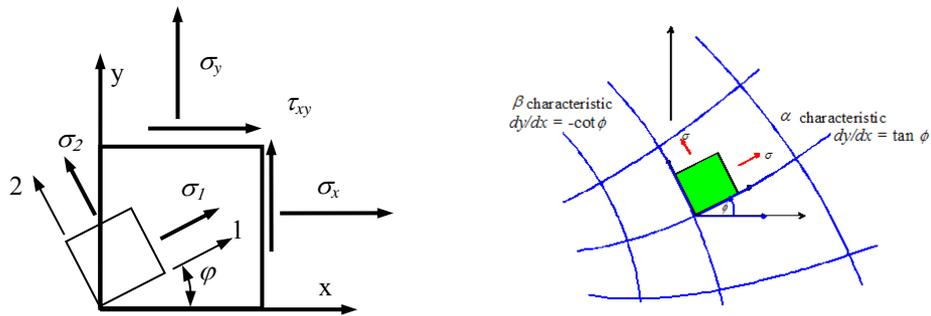
Fig. 1: Nomenclature in principal stress trajectories (left) and characteristic lines (right).
