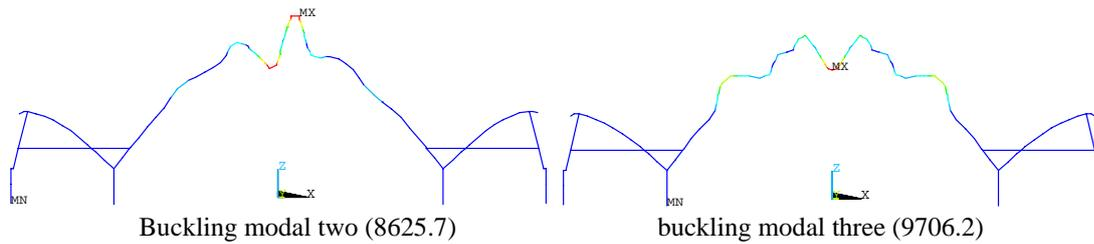
Figure.7 case 4 buckling mode
