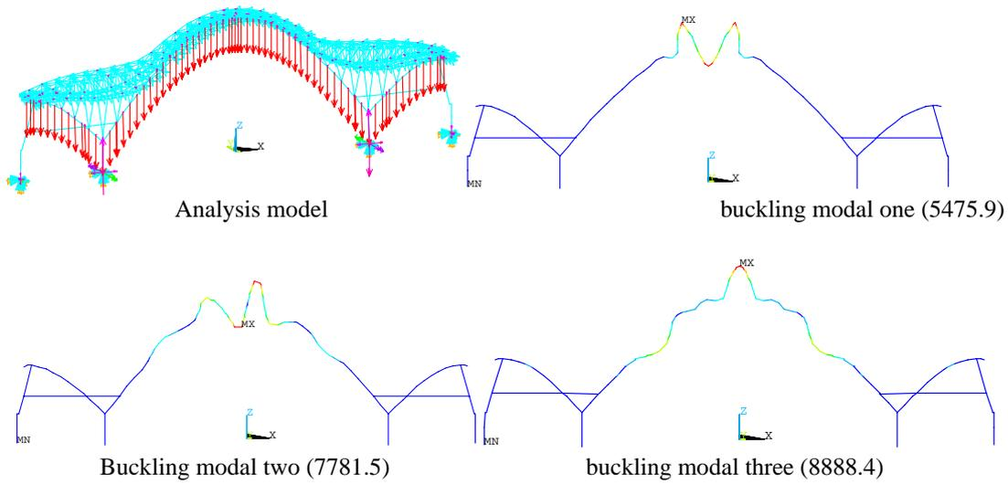
Figure.5 case1 buckling mode
