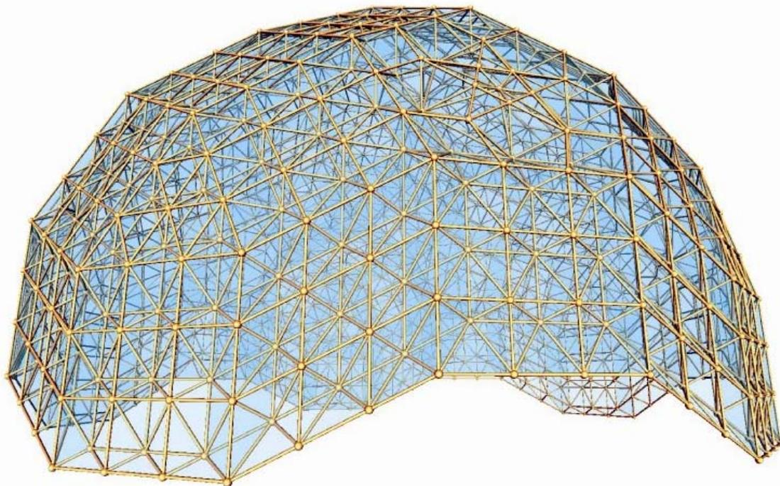
Figure 2: Any Golden Geometry skin model may be stiffened through a network of octet planes
