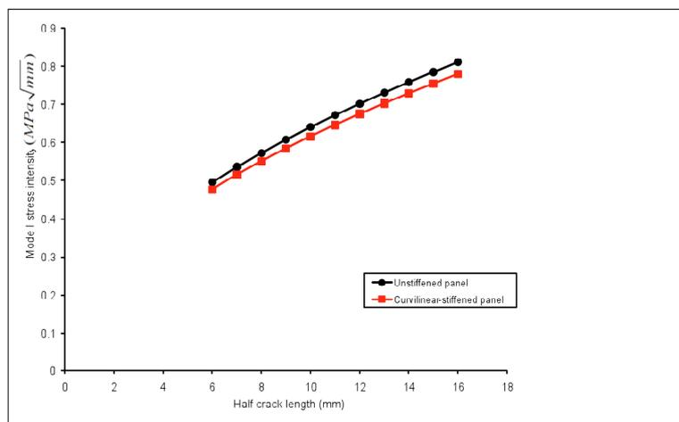
**Figure 7: Evolution of the mode I stress intensity factor versus crack length**
