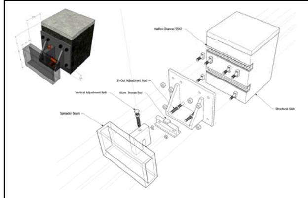
Figure 5: Anchor Bracket for Façade Panel
