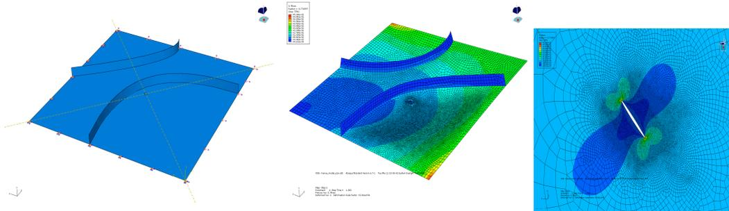
**Figure 6: Curvilinear-stiffened unitized structure panel under tension and shear loading, and cracked configuration**
