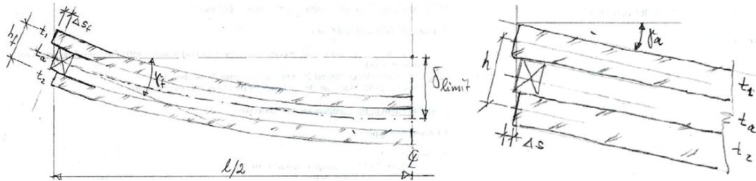
Figure 1: Compatibility of shear deformation and slope angle
