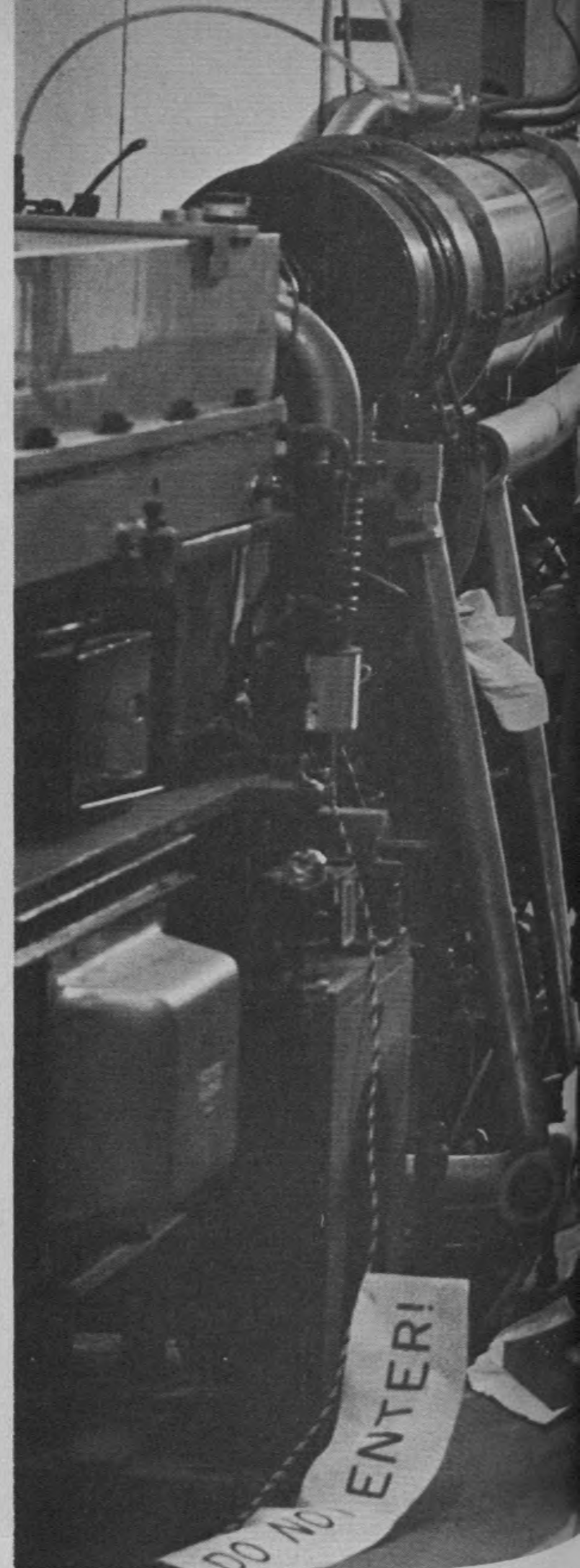
Linear accelerator (left) and radio frequency accelerators in the magnet ring (above, one of four) act in much the same way. Both push the electrons along on the crest of a wave, somewhat like a surfer riding a wave to shore.
