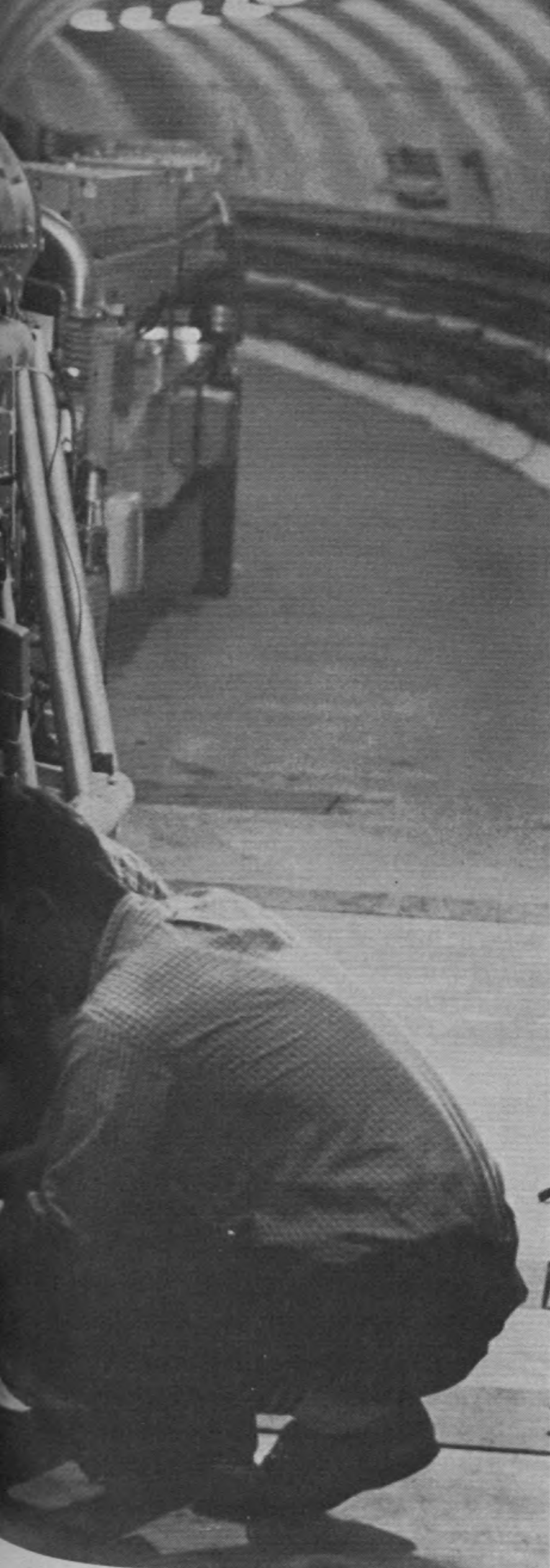
Where the magnet ring enters the experimental hall (right), researchers set up equipment to count, measure, and track the stream of particles that emerges from a collision between an electron or photon beam and a target nucleus.
