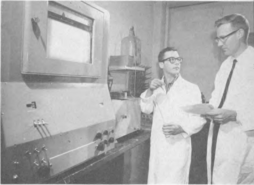
Professor McCormick and a graduate student use a recording spectrophotometer to measure changes in optical absorbcancy of coenzymes.
