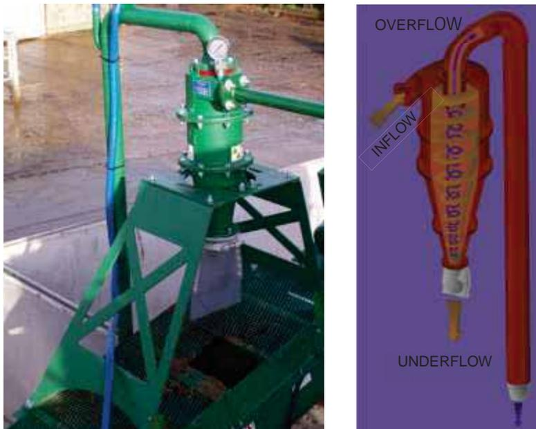
so a portion of manure solids settle as well (as illustrated in Figure 2). In the interest of preventing sand from filling digesters, this loss of organic matter is considered acceptable in comparison to the alternative, that being, decommissioning and removing solids from AD vessels.
