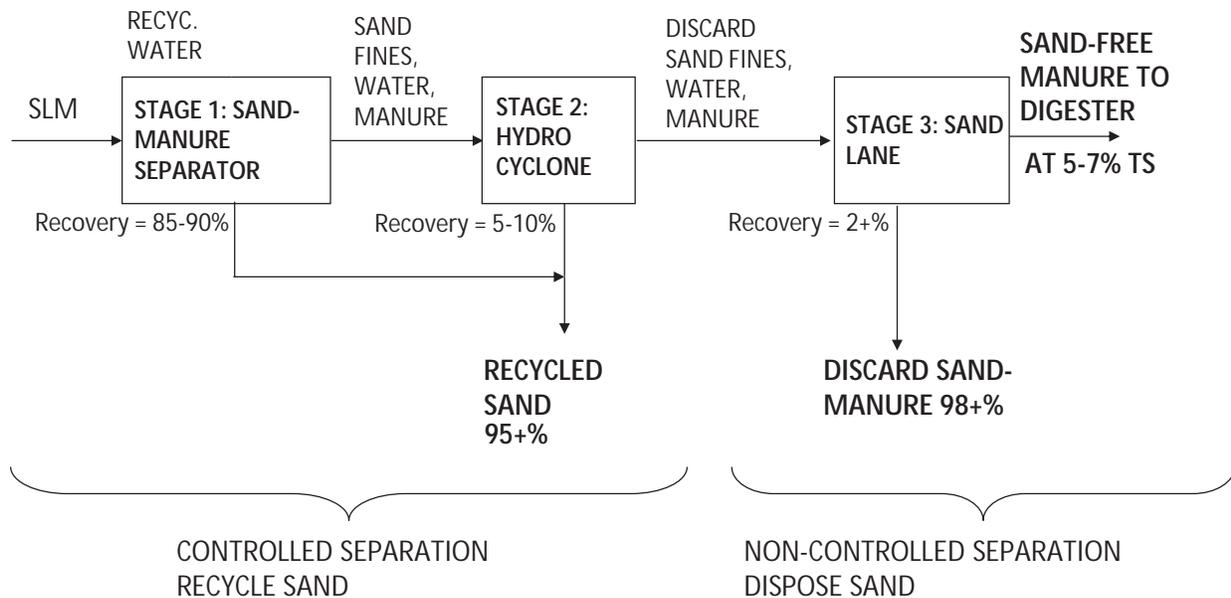
This primary phase of SMS achieves recovery of approximately 85 to 90%. The total solids content of the Stage 1 SMS effluent is approximately 5 to 7% TS. This corresponds to a dilution ratio of 1:1, or, one mass part of water to one mass part of SLM added to the system
