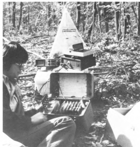
Electrical conductivity of the Earth's deep crust is measured at a field station in the Adirondacks as part of a graduate research project.
