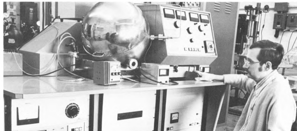
Above: Equipment in the Materials Science Center facility in Bard Hall includes this high-resolution Siemens 102 electron microscope used here by a graduate student in materials science and engineering. This microscope has provided images with line resolution of 2 angstroms.
