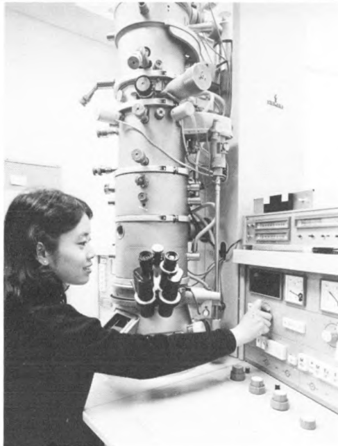
Above: Equipment in the Materials Science Center facility in Bard Hall includes this high-resolution Siemens 102 electron microscope used here by a graduate student in materials science and engineering. This microscope has provided images with line resolution of 2 angstroms.
