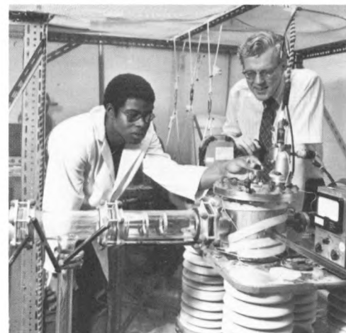
Above: This molecular beam epitaxial growth system is used to grow GaAs and related semiconductor materials for electronic devices. This research is directed by Professor Lester F. Eastman.
