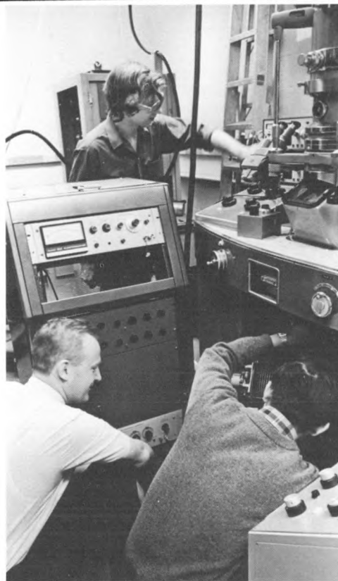
Professor John Silcox and students work with an electron microscope modified to include an electron spectrometer under on-line computer control.
