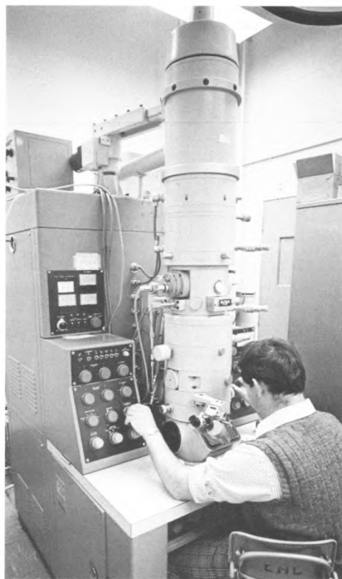
Electron microscope studies are among the projects available for Master of Engineering students. This instrument is a 200-keV electron microscope.
