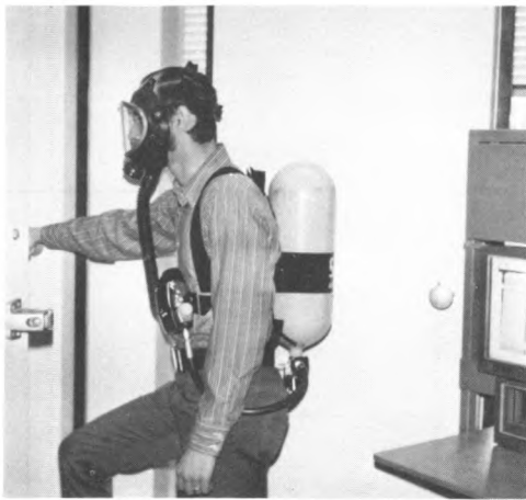
A researcher enters a controlled-environment chamber used in studies of optimal storage conditions for vegetables. The low oxygen levels are insufficient to sustain human life.
