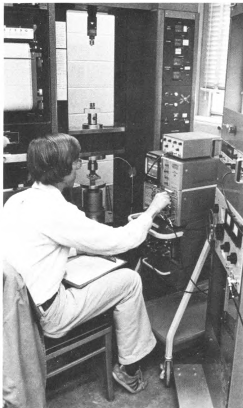
One facet of research in the nondestructive testing of materials is the use of ultrasonic waves to measure stresses in metal specimens under uniaxial loading.
