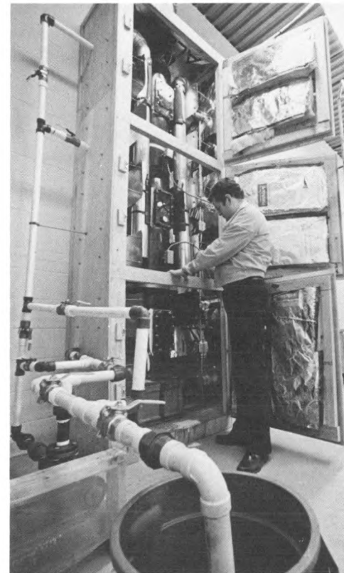
An experimental multipurpose reactor converts waste to three effluents: methane gas; solid float material, potentially useful for bedding or feed; and liquid, containing most of the nutrients, for fertilizer production.
