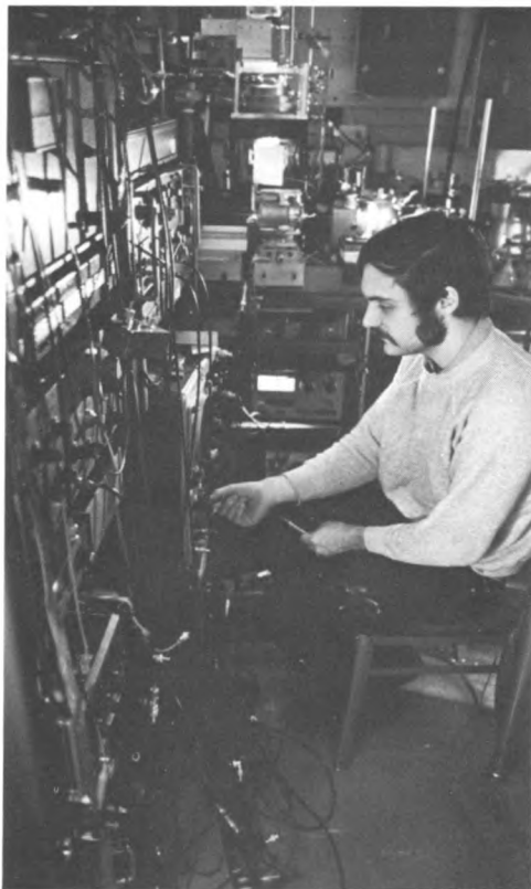
The kinetics of an important biophysical process are studied with use of a laser beam. Carbon monoxide bound to hemoglobin is "knocked off" by the beam and the speed of recombination is measured.
