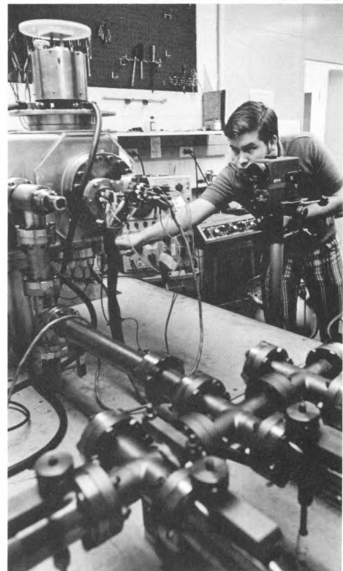
The inelastic scattering of electrons from single-crystal metal surfaces is used to study electron excitations in this ultrahigh-vacuum spectrometer.
