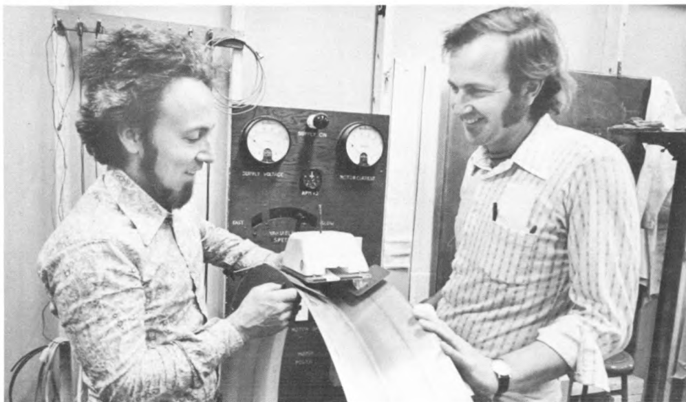
Professors Francis C. Moon (left) and Joseph A. Burns inspect a model of a magnetically levitated train.
