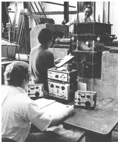
Above: Professor Richard White and graduate students are studying the strength of nuclear reactor containment vessels subjected to earthquake loads.
