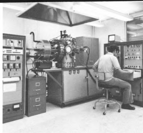
Above: This molecular beam epitaxial growth system is used to grow GaAs and related semiconductor materials for electronic devices. This research is directed by Professor Lester F. Eastman.
