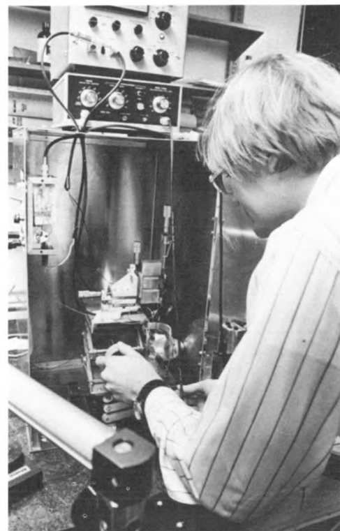
A study of nerve conduction processes is among the research applications of fluorescence correlation spectroscopy, a technique developed at Cornell. Here laser light illuminates fluorescent probes that indicate changes occurring when voltage is applied across an artificial membrane.
