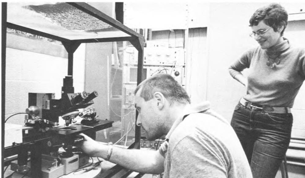
Voltage clamping of muscle cells is performed by Bruce Land, a postdoctoral associate of Professor Miriam Salpeter (standing) in research on the biophysics of nerve-muscle interaction.
