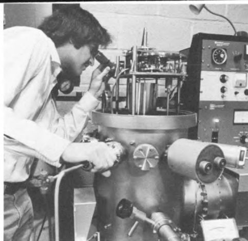
Equipment in the submicron facility includes a multiple-mask electron beam evaporation system for sequential deposition of patterned thin-film layers.
