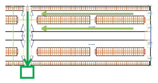
A flush flume system utilizes fast flowing liquid to transfer manure across the width of a barn or across several barns in a round tube. A high volume pumps creates an adequate flow rate to prevent settling of manure solids and bedding material. Water addition, and separation or dewatering is needed before evacuating to further processing to have enough liquid to keep the flush flume operating. Solids content of a flush flume will typically vary between 4 to 9% total solids.
